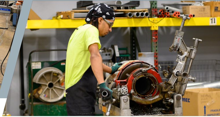
(Left) Ken Hotchkiss setting up the welding table for the next project. (Right) Apprentice Luis Cartagena threading conduit for the Willard Day Treatment Project.
