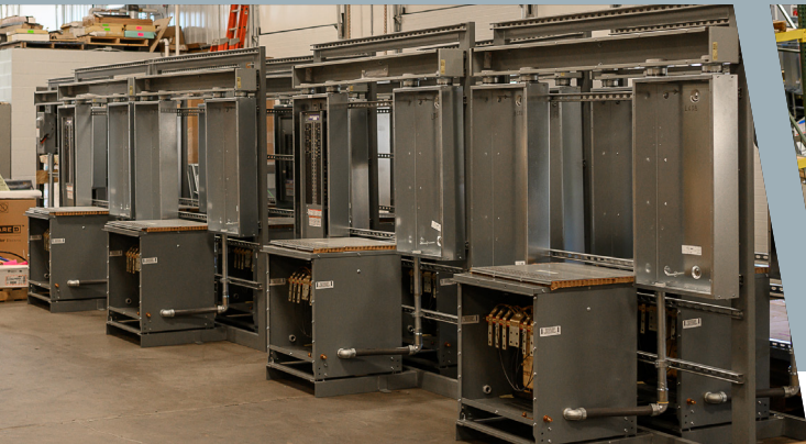
(Left) Panel, transformer and panel equipment awaiting panel interiors and transformer wiring for the Amazon Project. (Right) Jeff Veers and Dave Wilkins assembling inmate radios for the Auburn Correctional Facility.
