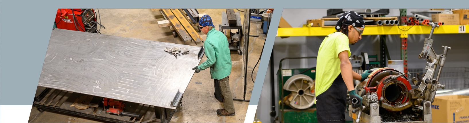
(Left) Ken Hotchkiss setting up the welding table for the next project. (Right) Apprentice Luis Cartagena threading conduit for the Willard Day Treatment Project.
